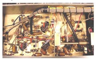
The IF/AF chassis during component replacement (annotated photo at the end of the article, Page 24)
