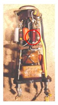
Inside the BFO unit – note C100 (10uf electrolytic) lurks in here (circled)
