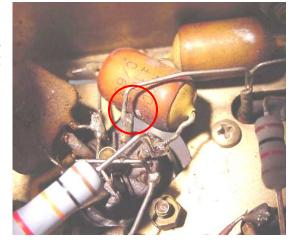
Lead from T4 secondary/C88 where it was pressed hard against the case of C82 (note small 'bare' spot' where it had been resting)
