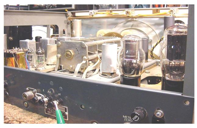
A nice shiny new 5Z4G fitted and not an electron to rectify...
