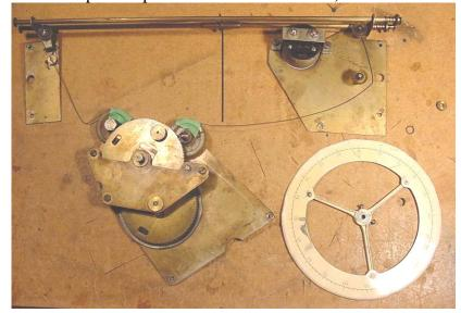
from all angles for reference. The drive cord looked in reasonable condition, so I decided to leave it fixed to the spool pulleys at either end and to remove the assembly intact – hoping that I would not have to re-string the dial (see EUG Newsletter #25, p17 for tips on this if you have to do it).
