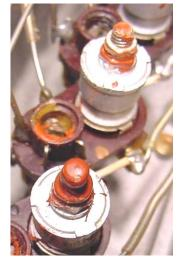
Hardened red sealing wax on the concentric trimmers and coil slugs
