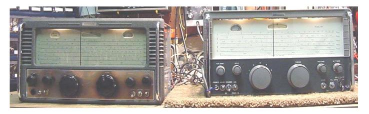
The S.940 on 'soak test' powered by the S.770R
