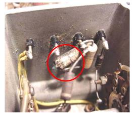
Burned-out R9 (not) feeding HT to V1
