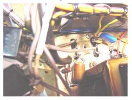
First I removed the can from the BFO unit and did some cursory component and pin-out checks before refitting it to the chassis and re-wiring into the circuit. While I had the opportunity I checked C72 (metalised paper heater decoupler) and found it to be leaky – replaced it (blue capacitor in photo, left).
