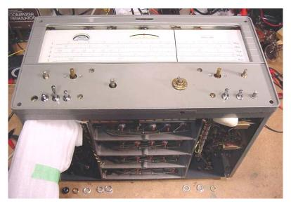
the controls in place while you fit the retaining nuts (saves a lot of time and cursing).
