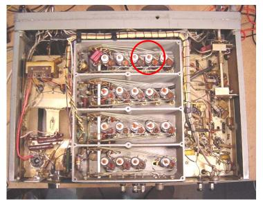
GZ34 (or 5Z4G) rectifier. The 5U4G tested ok, but should not be used in this application (even though it has the same pin-out) as it takes an extra amp of heater current and has a
